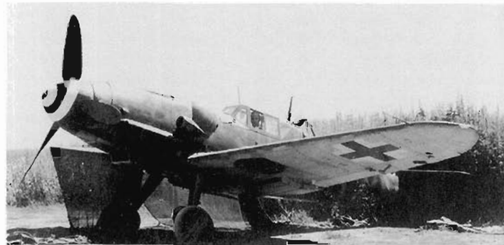
ABOVE: The positioning of the underwing Balkenkreuz was slightly further outboard as noted, but the undisturbed background paint, indicates that the original 76-colouring had been retained. (NASM via Dr. J. H. Kitchens & J. R. Beaman)
