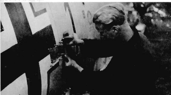
ABOVE: The amount of repair work able to be carried out at front line-level was relatively limited. Here, a ground staff member of III./JG 26 was photographed while applying a metal patch to the inside surface of the fuselage of a Bf 109 E, having already carefully removed a rectangular section of damaged metal. The pressure clamps further out from the hole define the real size of the metal patch.
