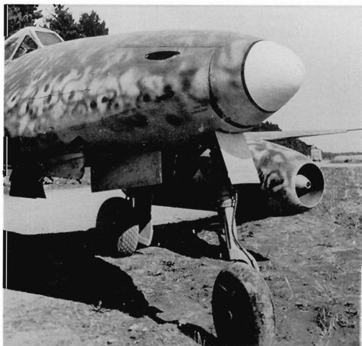
ABOVE AND BELOW: Three photographs of Me 262 A-2, 9K+YH, of 1./KG 51, showing the difference in style of the two production line painters who had camouflaged the aircraft. The port side had soft mottles while the starboard side had a more linear form of application. The nose cone was white, the Staffel colour, the same colour being added to the tip area of the fin and rudder. The style of the aircraft letter 'Y' was most unusual, having a cursive form with a curved lower stroke. Overall camouflage was 81/82/76.
