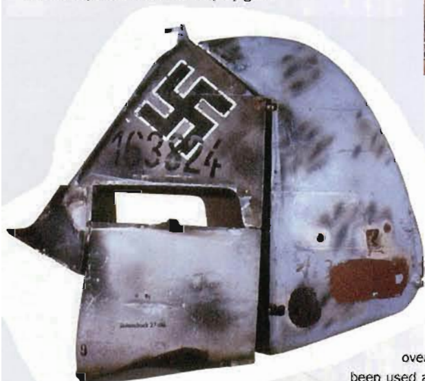
ABOVE: A close-up detail of the sprayed 83 on the rudder showing the coarse application caused by using too low a pressure with the spray gun.
