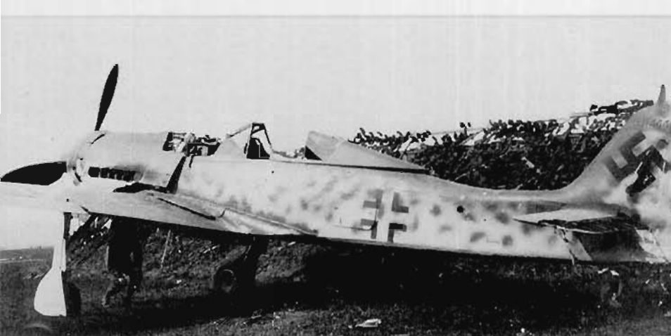
LEFT: Somewhat more consistent with camouflage patterns, if not always the colours used, were the late war piston engine fighters. Fw 190 D-9, W.Nr. 601444, had standard 74/75/76 finish with a solid application of the darkest colour forward of the canopy. The shattered canopy has exposed the 66-coloured, elongated headrest. (P. Miller via M. Olmstead)
