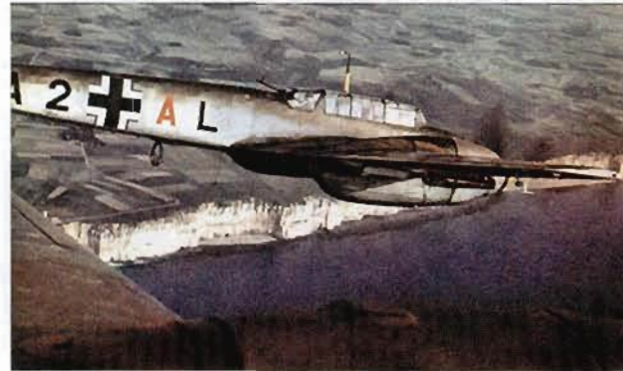
ABOVE: This in-flight view of a Bf 110 C of II./ZG 2, A2+AL, shows the application of a fine spray of 02 over part of the upper surface camouflage, markedly toning down the effect of the segmented 71/02 pattern along the spine of the fuselage.
