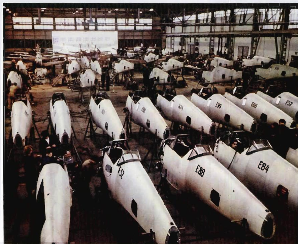
ABOVE: Bf 109 E-4s undergoing final painting. The two in the foreground still have wings painted in 02 with the fuselage in overall 65. The sub-contracted tail units however have 71/02 camouflage. Behind is CA+PG, in full camouflage. The aircraft behind have '159', '200' and '300' roughly marked on each engine cowling, possibly the last three digits of their Werknummer. The black '1' and '5' markings on the aircraft in the foreground may have been flight test numbers.
