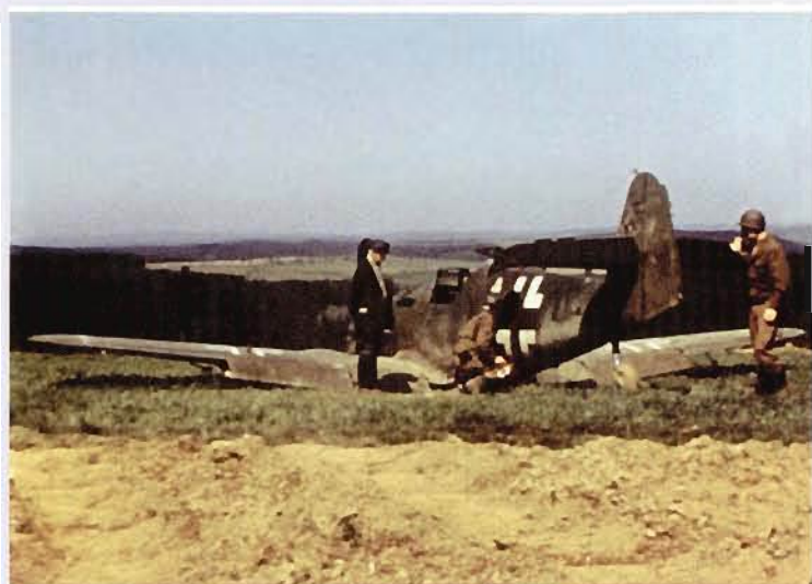
BELOW: The second aircraft to crash-land was 'White 8', also a 1. Staffel machine, and presumably from the same Jagdgeschwader. A Bf 109 K-4, it had a camouflage that appears to be of darker combination, possibly 81/83. The lower side surfaces of the fuselage were 76, but again the yellowish mud thrown up during the belly-landing has added a yellowish colour to the undersides. Again the aircraft lacked any Reichsverteidigung markings. (J. Crow)
