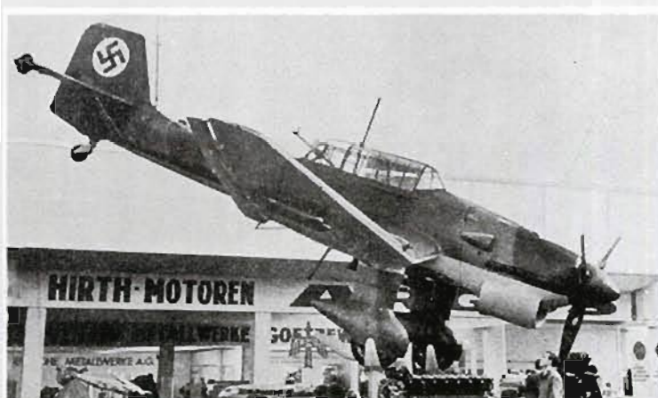
ABOVE AND RIGHT: Two views of the Ju 87 B displayed at the Brussels Air Show in 1939. The colours were 61, 62, 63 for upper and side surfaces with 65 for the under sides. The pattern used was quite unique, using soft and in places, slightly curved, lines of demarcation. The undercarriage spats were 'split' vertically with 61 at the leading edge and 62 for the rear half. This was the first time the type had been publicly displayed at one of the major Western air shows of the period, but examples had already been sold to pro-German allies to the east.
