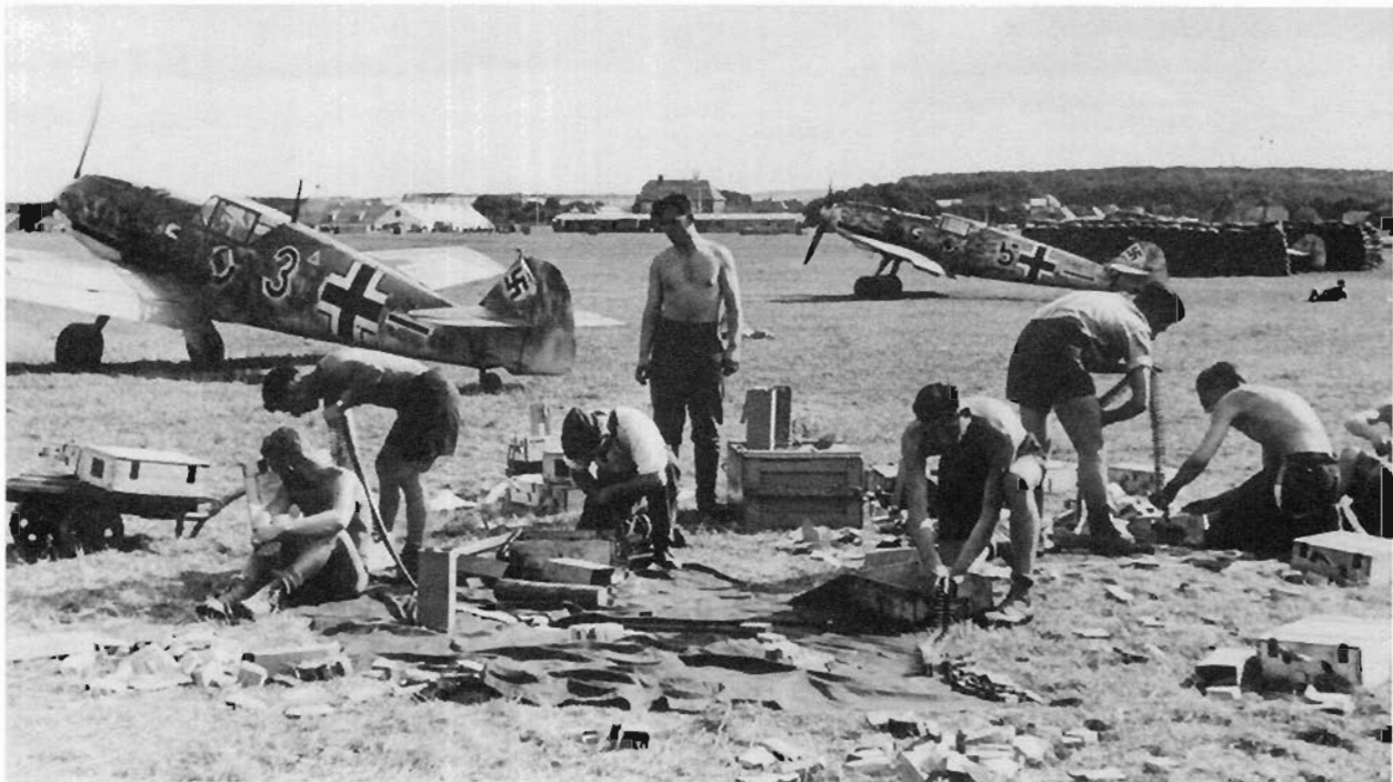
LEFT: A similar style of application had been applied to this Bf 109 E-4, 'Yellow 5', camouflaged in standard 71/02. In this case 71 appears to have been used as short dashes of colour over a very thinly sprayed finish of 02 on the fuselage side surfaces; some of the 02 had also been applied over the spine of the aircraft. Note the high contrast around the square of the Hakenkreuz marking, part of the original standard 65-background. Wing and horizontal tail surfaces however remained in plain 71/02 finish. The rudder was finished in white, indicating that the photograph was in September 1940. (F. Kovács.)
