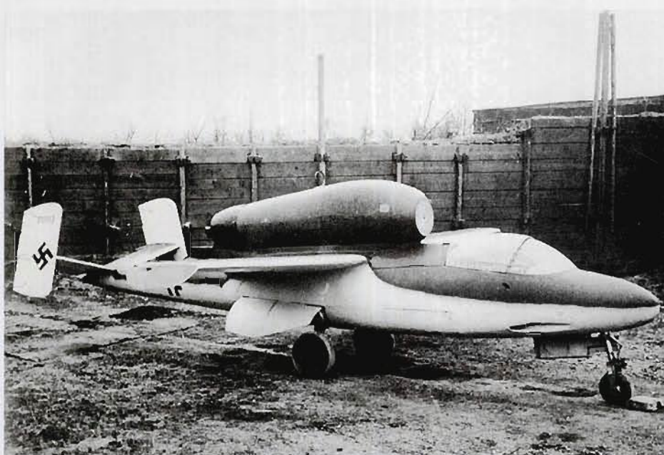
LEFT: The third Junkers-built He 162 A-2, W.Nr. 310003, produced in late February/early March 1945, and armed with two MK 108 30 mm cannon. The diminutive airframe of mixed wood and metal construction resulted in the type being camouflaged on all surfaces despite austerity measures then in force. Although the official painting schedule for the type called for an 81/82/76 scheme, upper surface camouflage here was the low contrast 81/83, with possibly green-blue lower surfaces.
