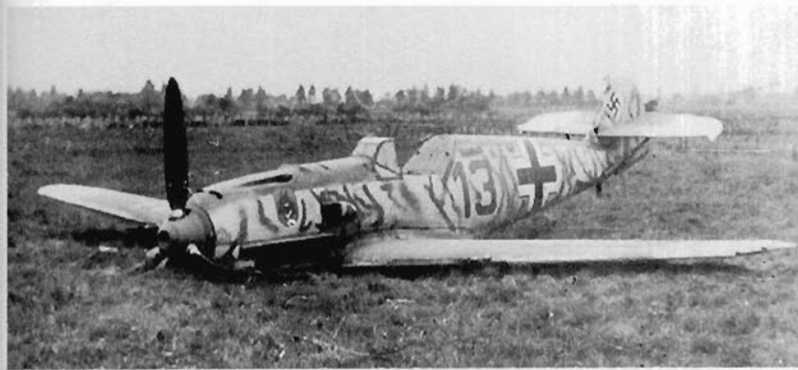
RIGHT: Bf 109 Es of 1./JG 3 seen in October 1940 illustrate another form of amended camouflage, this time using a soft spray of 02 on the flanks with soft mottling in 71. The engine cowling and rudder were both painted in 04 yellow.
