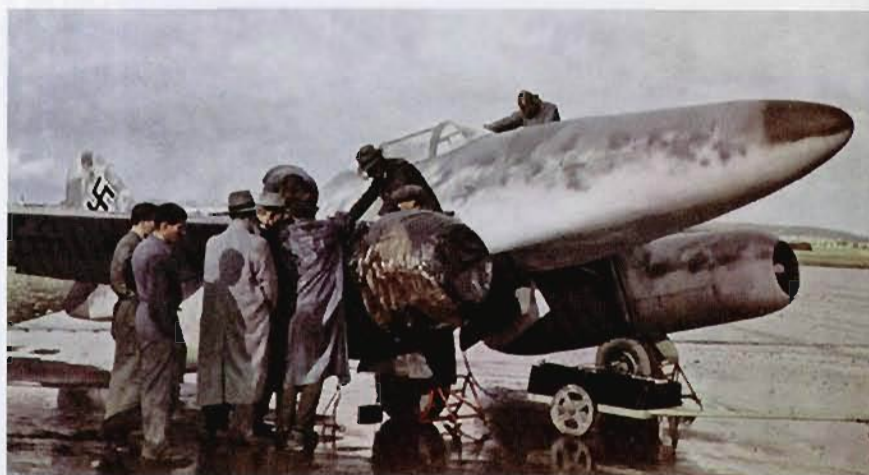
ABOVE: The Me 262 V-3 was first flown in early 1942 and as such carried standard fighter camouflage for the period – 74/75 with a slight mottling in both colours applied to blend upper and side surface colour transition. The nose cone was finished in 70, probably to give the impression of a conventional spinner to prying eyes. The engine cover was finished in ground defensive camouflage of brown and black, the same RAL colours used for the wheel covers.
