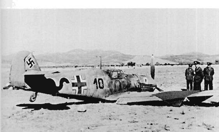
ABOVE: A Bf 109 E-3 of III./JG 77 brought down during the Balkans campaign. Camouflage was 71/02 with fuselage side surfaces mottled with softly sprayed 71 and 02 that almost obscured the 65-colouring in many places. Note the stronger contrast between the 71 and 02 on the section of the wing outboard of the cloth draped over the Balkenkreuz marking. Tactical markings were 04 on rudder and engine cowling. The 9. Staffel badge below the cockpit had been discoloured by the engine exhaust, but the III. Gruppe marking on the cowling is clearly visible; note the latter large style. The aircraft retained the 1939-size Balkenkreuz marking and smaller code application, the numeral size being based on the proportions of the Balkenkreuz.
