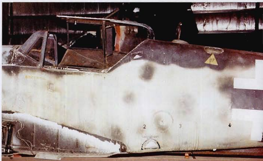
LEFT AND BELOW: The main fuselage of W.Nr 163824 showing the green-blue side surface colouring that contrasts markedly with the 76-coloured engine lower cowling. The brown-violet colouring on the nose section, and above the Balkenkreuz marking stands out against the black-grey colouring. Cockpit framing is in standard 66. The recycled ammunition bay top cover has its original 78 tropical blue colouring exposed where the black-grey colour has been scuffed off. (K. Ginnane)
