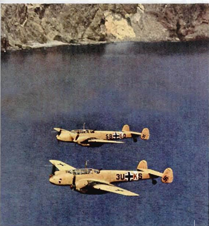
ABOVE: These two Bf 110s of ZG 26 flying over the Mediterranean clearly show how RLM 79 Sandgelb alone stood out against the blue water.
