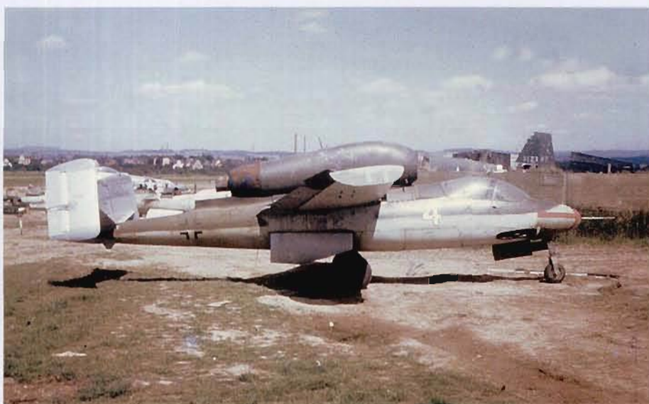
RIGHT: A rare colour photograph of an He 162, 'Yellow 4', W.Nr. 120067, of 1./JG 1 showing the 81/82/76 scheme. The final painting instruction for this type had set down a system of component colouring, rather than the usual random shape pattern in the two upper surface colours. However, close examination of this photograph, and also a black and white photograph of the same aircraft, taken at Leck in May 1945, show that the 81 and 82 had been applied in the old standard style. The entire tail plane section had been replaced, the original one, bearing the Werknummer in white and a white outline-style Hakenkreuz, had both surfaces of the fin and rudder assemblies in full camouflage. Note the large area of red oxide metal primer on the tail cone of the engine, showing the poor adhesion of the baked black stoving enamel finish used for this heat sensitive component. (S.Coates)
