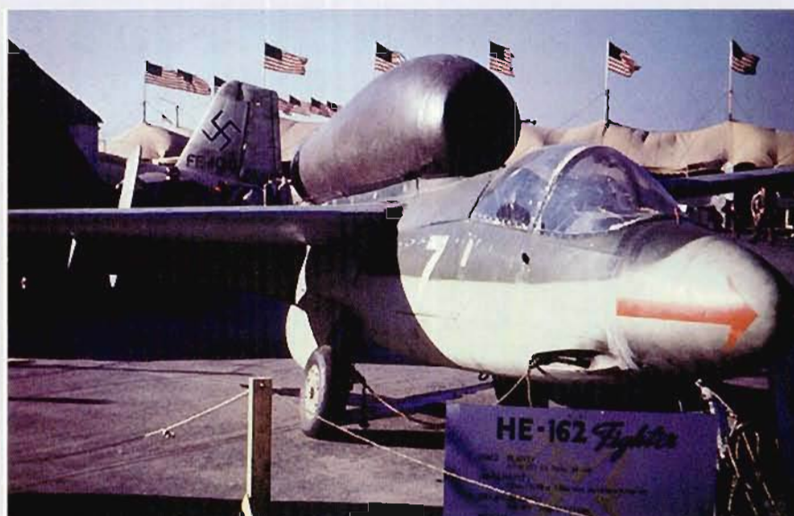
RIGHT: Another well colour balanced photograph of an He 162 A-2 on display post-war. The 81/82 upper surface colours can be determined as well as the green-blue lower surface colouring. Compare the latter with the intense blue of the sky. By the time this aircraft had been built, 76-colouring had been reduced to a greyish-white colour with only a touch of blue in it.
