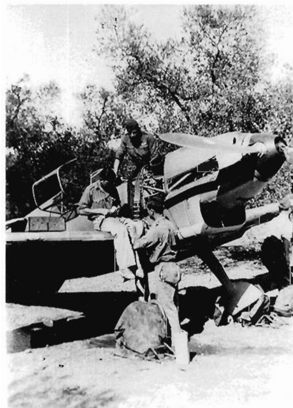
RIGHT: The distinction between the 62 and 65 colouring can be more clearly seen in this close-up of ground staff rearming a Bf 109 D-1. Note the canvas wheel cover, camouflaged with RAL 8019 (RLM 61 and RAL 6003 (RLM 62) colouring. (D. Vincent)
