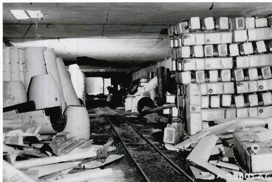
RIGHT: The chaotic conditions in the Me 262 parts storage facility at the Obertraubling plant were indicative of this industry as a whole. With the exception of the fuel tanks, the remaining items were all pre-painted in 76. Engine cowling parts, all undercoated in 02, are stacked on the left while to the right are leading edge slat units undercoated in 02. In the latter case this was required by the RLM as they were steel units and had to be given some anti-corrosion covering during storage and distribution though even that protection was eliminated in some instances. All were sub-contracted parts.
