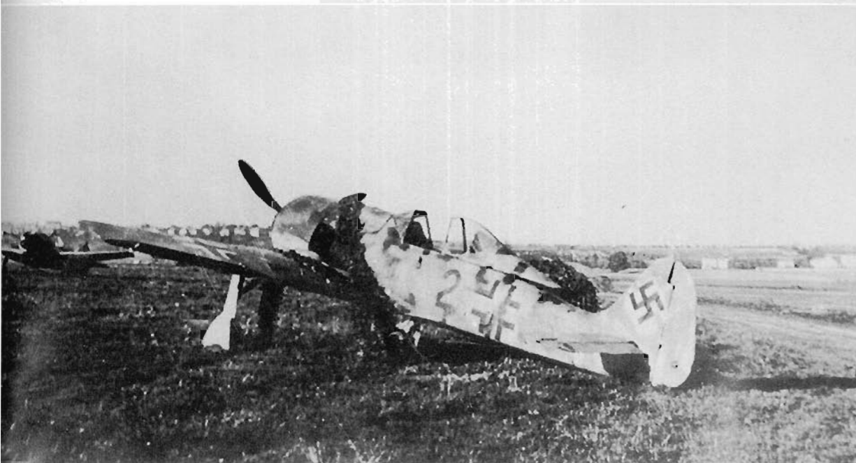
LEFT: A most unusually modified camouflage. The fuselage of the Fw 190 appears to be finished in a base coat of 82 with long thin patches of 81 added in semi-linear fashion. The fin and rudder lack anything but the 82-colouring, but around the Hakenkreuz the original 76 can still be detected. In contrast the wings and engine cowlings appear to be in very dark colours; possibly a much denser application of 81 and 82. (J. Crow)
