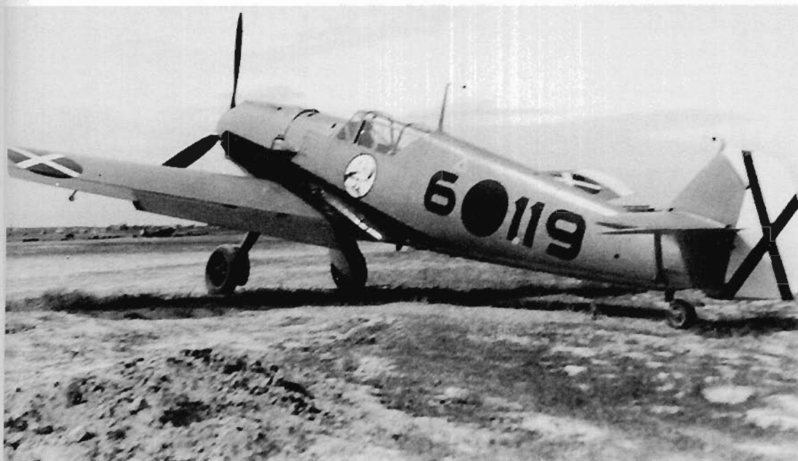
ABOVE: This rear angle view of Bf 109 E, 6-119 shows the full extent of the black trim marking introduced to screen the dark stains from the engine exhausts on the 62-green of the upper surface camouflage. This was the mount of the last Staffelführer of 1./J 88, Hptm. Siebert Rents, and was amongst the batch of Bf 109 Es handed over to the Spanish Air Force at the end of hostilities in Spain.
