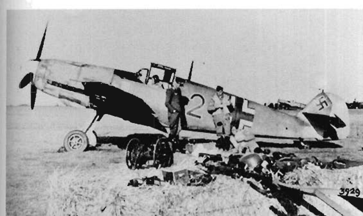
ABOVE: Early deliveries of the improved Bf 109 F series in September 1940 carried standard 71/02 with mottling applied to the fuselage side surfaces. This aircraft had its side surfaces almost covered with a light spray of 02 taken right down to the lowest point. Based on the French coast, yellow tactical markings have been retained for engine cowling and rudder. The temporary yellow on the engine cowling tended to deteriorate more quickly than that applied to the rudder, heat from the engine no doubt hastening the process sometimes producing a deeper shade of colour.
