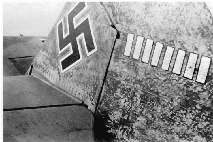
ABOVE: Close detail of the application method used by JG 2 for some of its aircraft. The stipple effect on W.Nr. 5274 was produced by using a 'stabbing' motion with one of the larger size brushes from the standard painter's kit issued as maintenance equipment. This style of finish has often been erroneously identified with use of sponges, an item that was not part of the standard kit. The series of repetitive near half circle shapes at the base of the fin show that the edge of a circular brush had been used. (E. Mombeek)
