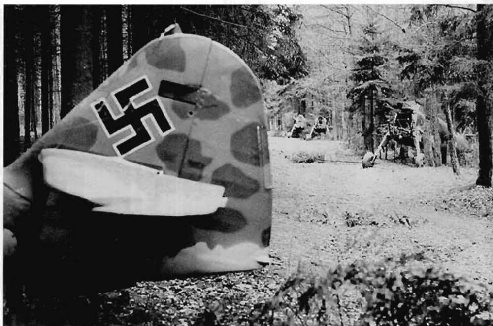
RIGHT: Not the same aircraft as in the previous photograph as close examination of the positioning of the spots of 83-colouring show (see the lower rearmost spot of 83). These aircraft were all found near Wertheim. The near consistency of their shapes and the bottom colour division line makes it clear that a stencil had been used. The unpainted area below the fixed horizontal tail surfaces and bare metal rear access panel can also be seen. However, note the dark 81-coloured rear section of the fuselage with that colour taken up over the fin fairing. The remainder of the fuselage was 82/83. Compare these two photographs with that on page 42 of the stockpile of Bf 109 fins that had free-hand applied camouflage.
