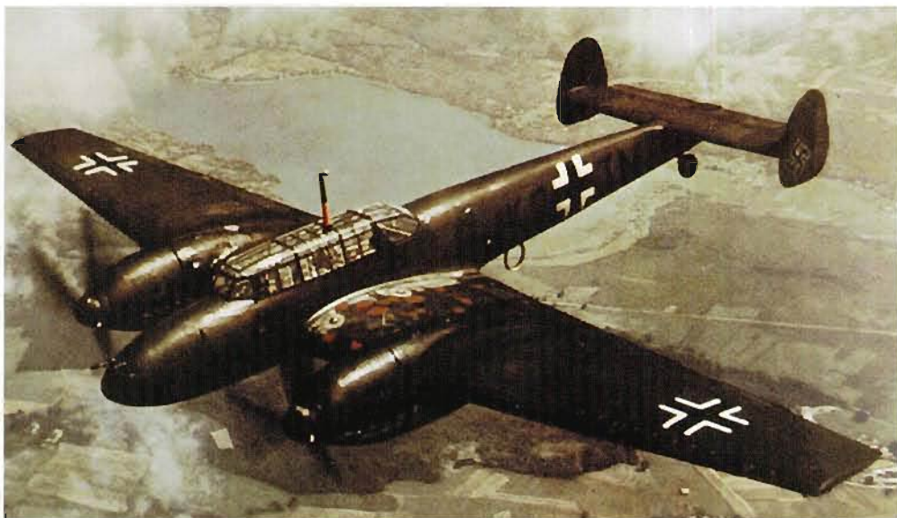
ABOVE: Bf 110 C W.Nr. 2143 KD+TM in factory-finished splinter camouflage of standard 70/71/65. Some small patches of red oxide primer can be seen on the wing root walk area. This aircraft was test flown on 17 May 1940.
