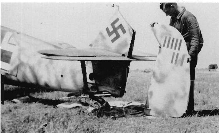
ABOVE: The amount of repair work able to be carried out at front line-level was relatively limited. Here, a ground staff member of III./JG 26 was photographed while applying a metal patch to the inside surface of the fuselage of a Bf 109 E, having already carefully removed a rectangular section of damaged metal. The pressure clamps further out from the hole define the real size of the metal patch.
