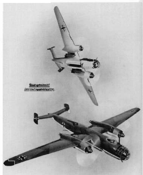
ABOVE: This advertising poster for the Fw 191 A bomber, based on Focke-Wulf's advertising scale model of the aircraft, illustrates the standard camouflage pattern in 70/71/65 that had superseded the old three-colour upper surface scheme by 1938.
