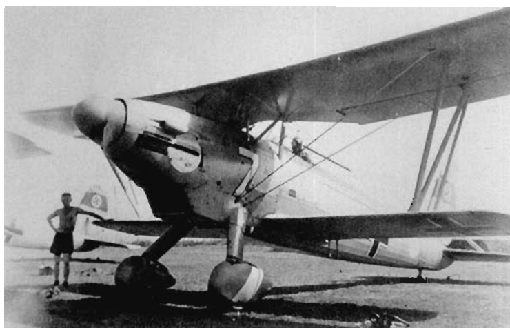
ABOVE: In Germany, prior to the appearance of the Bf 109 Bs, Ar 68 F-1 fighters had replaced He 51s, initially retaining the contemporary 63-overall colour scheme as seen here on this 3./JG 134 aircraft. Upper decking of the fuselage was in mid-range colour, possibly RLM 24. 'White 7' was the mount of Otto Hintze. (Hintze via J.Vasco)
