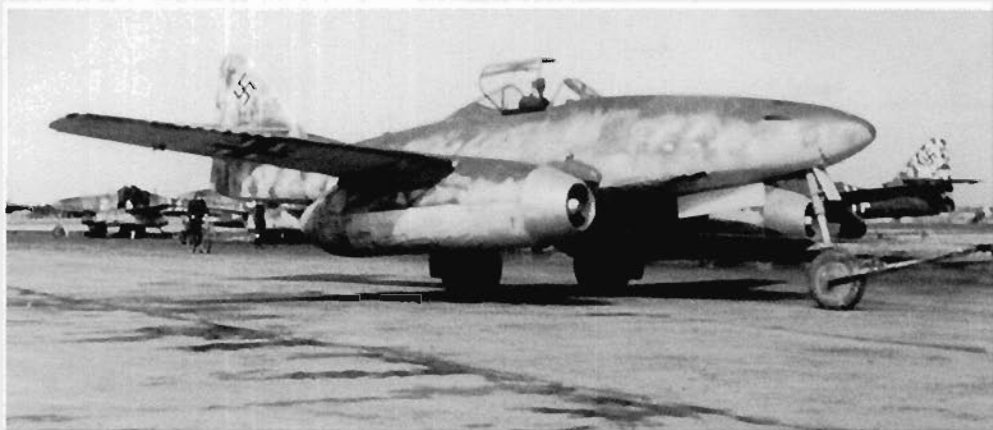
ABOVE: W.Nr. 110813 as 'Green 3' in service with Kommando Nowotny. Note that by then both engines had been replaced with the front section of each engine, which formed part of the engine as delivered, being left in bare metal finish.
