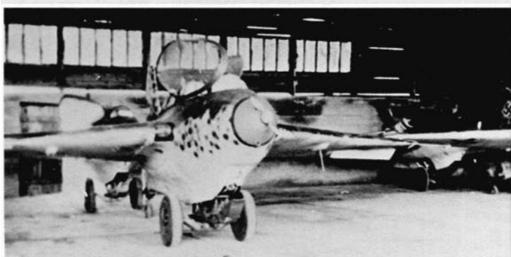
LEFT: The diminutive Me 163, of mixed wood and metal construction, received full camouflage despite the austerity measures. Issued to JG 400, this particular machine wore an 81/82 camouflage with spots of both colours applied to the nose area. The nose cone was 04 with a 23 coloured line dividing it from the camouflage.
