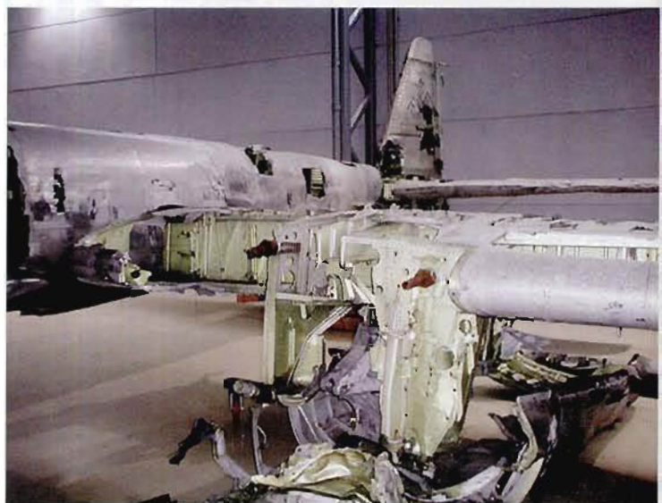
ABOVE: The same anodised finish was used for the Ju 88 and testimony to its durability is this photograph of a Ju 88, recovered from the sea in only recent years. It is now on display in the Flymuseet in Norway. The resistance to corrosion of this finish is evident. (Flymuseet)
