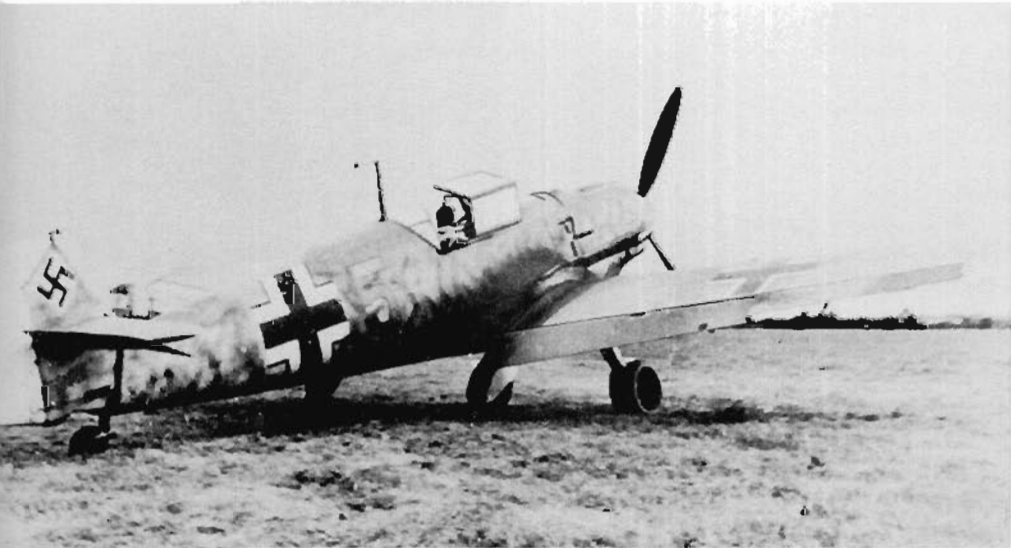
LEFT: A similar style of application had been applied to this Bf 109 E-4, 'Yellow 5', camouflaged in standard 71/02. In this case 71 appears to have been used as short dashes of colour over a very thinly sprayed finish of 02 on the fuselage side surfaces; some of the 02 had also been applied over the spine of the aircraft. Note the high contrast around the square of the Hakenkreuz marking, part of the original standard 65-background. Wing and horizontal tail surfaces however remained in plain 71/02 finish. The rudder was finished in white, indicating that the photograph was in September 1940. (F. Kovács.)
