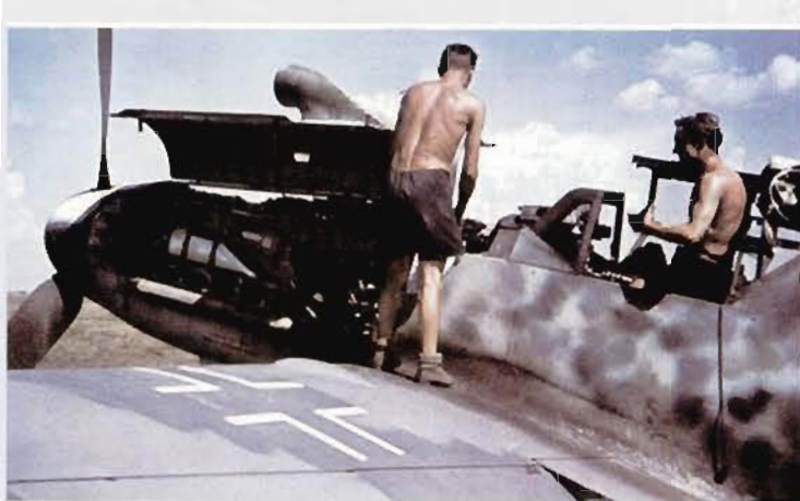
ABOVE: This Erla-built Bf 109 G-6, 'White 10', W.Nr. 19881, flown by Lt. Willmans of 1./JG 52, shows the mix of mottle colouring to the fuselage side surface in colours 74, 75 and 02. (M. Jessen)
