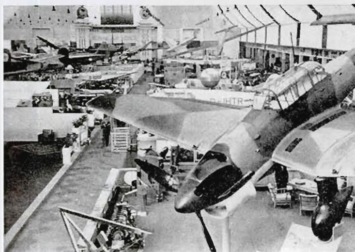
ABOVE AND RIGHT: Two views of the Ju 87 B displayed at the Brussels Air Show in 1939. The colours were 61, 62, 63 for upper and side surfaces with 65 for the under sides. The pattern used was quite unique, using soft and in places, slightly curved, lines of demarcation. The undercarriage spats were 'split' vertically with 61 at the leading edge and 62 for the rear half. This was the first time the type had been publicly displayed at one of the major Western air shows of the period, but examples had already been sold to pro-German allies to the east.
