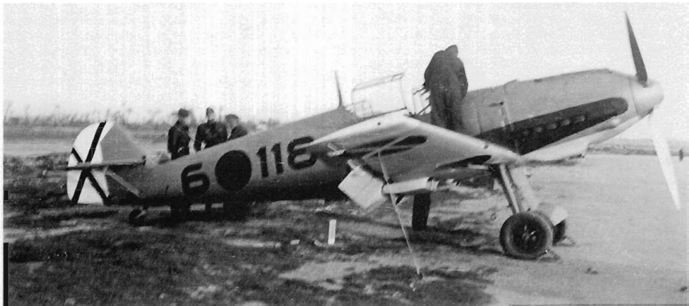
ABOVE: Bf 109 E-1, 6-118, one of 45 delivered to Spain, photographed in 1938, illustrates the universal 62/65 camouflage that had been adopted for the Bf 109 force by late 1937. Use of stylised black trim for the exhaust area and wing root fillet was a feature introduced with deliveries of the 'E' variant.
