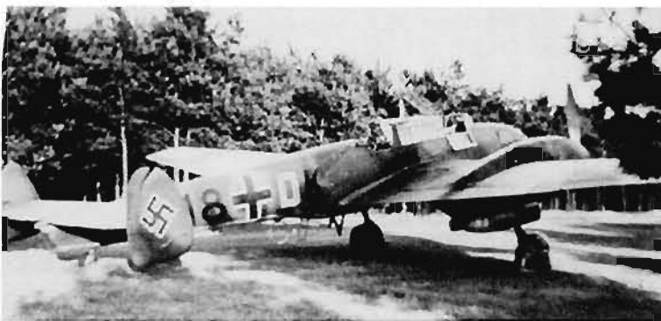
ABOVE: Bf 110 C M8+DK of I./ZG 76. was photographed during the Polish campaign. The 70/71 camouflage can be seen, but the effects of lighting conditions could make it difficult to discern. The individual letter was painted in the 2. Staffel colour of red and outlined in the Gruppe colour of white.
