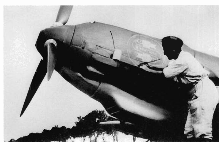
ABOVE: A range of painting equipment was issued to units for general minor maintenance and marking of such items as aircraft identification numbers and Staffel markings, etc. as seen here – a personal emblem of one of the JG 53's pilots being painted using a 1.25 litre tin, balanced on the exhaust stub shield, and one of the smaller of the round brushes. (Eric Mombeek)
