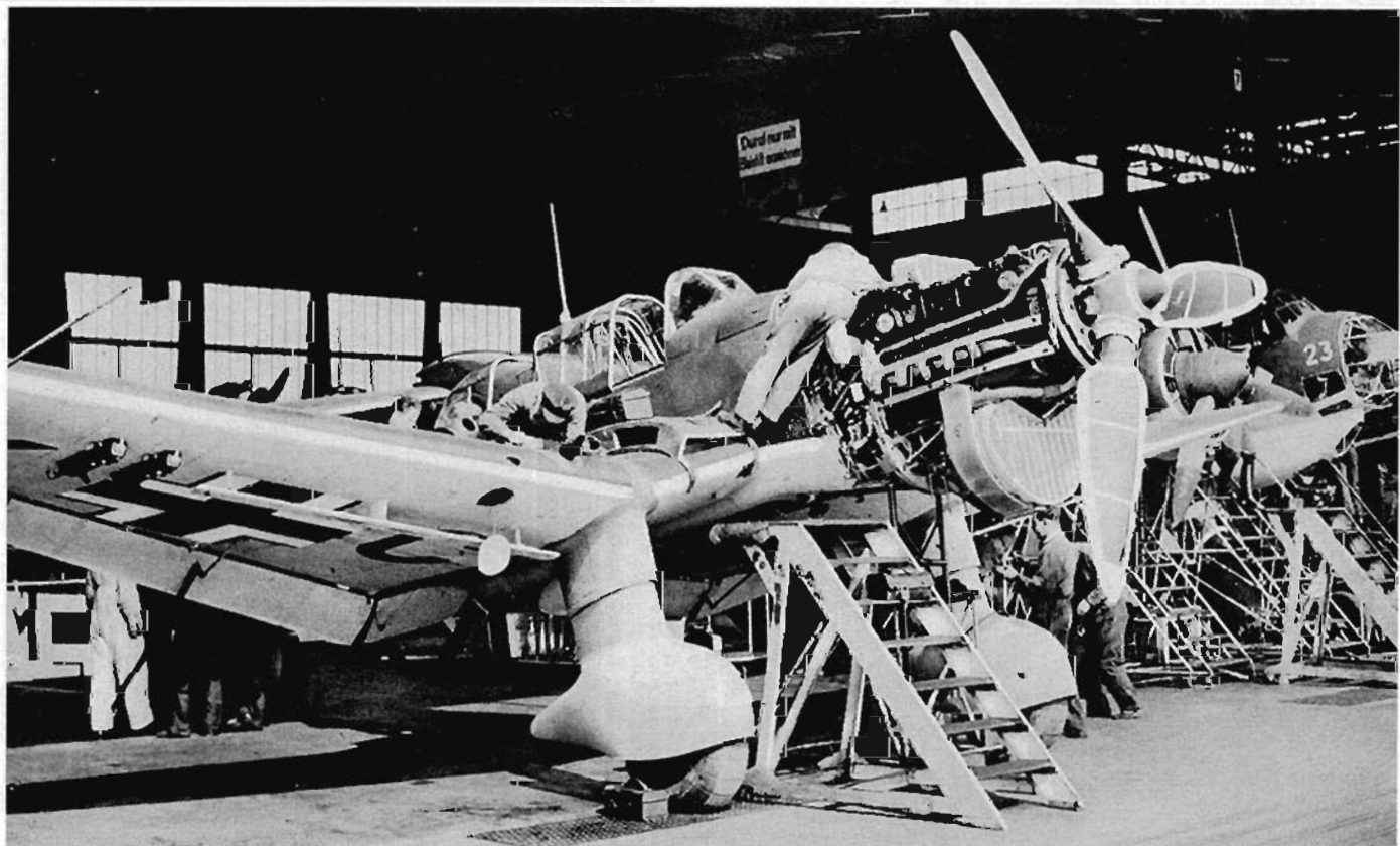
BELOW: The finished aircraft was rolled out for a final check of engine and ancillary services. The protective padding on the lower two propeller blades remained in place until the aircraft was ready for transfer for its factory acceptance test flight. The first two letters of the Stammkennzeichen on the machine were XO, and the size and positioning of the underwing Balkenkreuz marking indicate that this was probably part of the 1939/40 production cycle.
