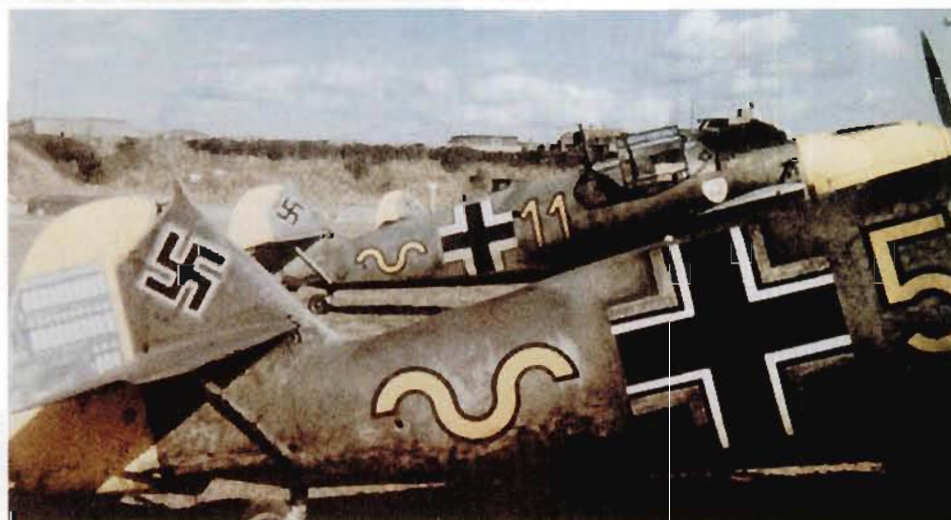
ABOVE: Close detail of the application method used by JG 2 for some of its aircraft. The stipple effect on W.Nr. 5274 was produced by using a 'stabbing' motion with one of the larger size brushes from the standard painter's kit issued as maintenance equipment. This style of finish has often been erroneously identified with use of sponges, an item that was not part of the standard kit. The series of repetitive near half circle shapes at the base of the fin show that the edge of a circular brush had been used. (E. Mombeek)
