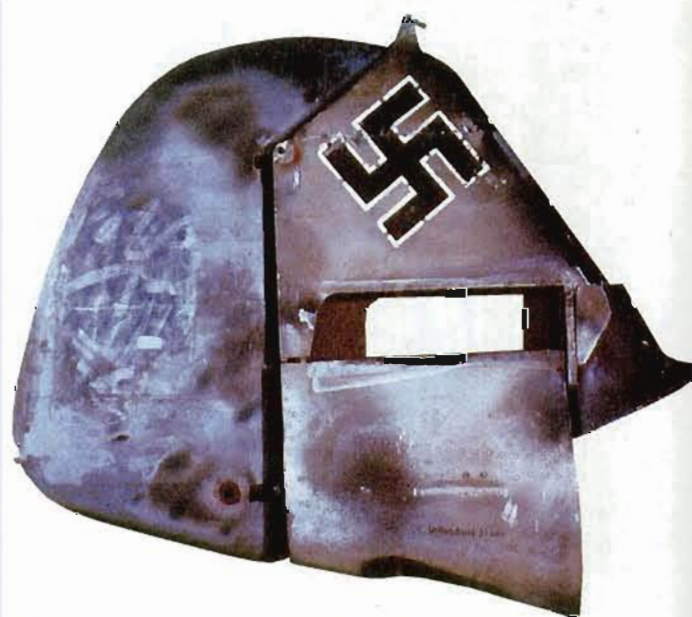
LEFT AND RIGHT: The tail unit, a complete sub-component, in this case a recycled one from a Bf 109 F, and a recycled rudder. A strong overspray of 02 had been used as camouflage above
