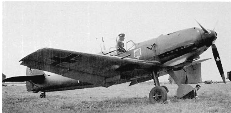
ABOVE: This Bf 109 E-3 of I./JG 76 (later II./JG 54) also appears to have a monochromatic finish. However, careful examination of the wing leading edge reveals the presence of a two-tone pattern with segments that correspond to a Type 2 pattern. The style and positioning of national markings and the Hakenkreuz clearly date this photograph to post-January 1939.
