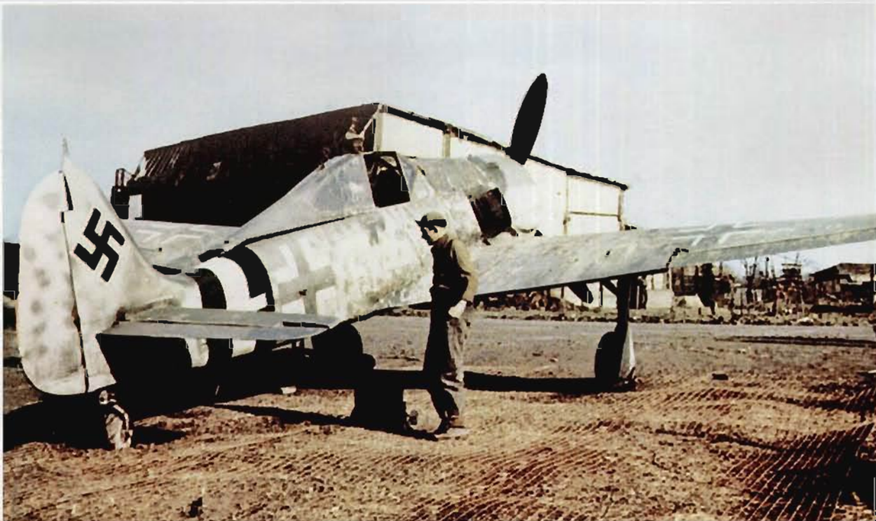
LEFT AND BELOW: These two colour photographs of the same aircraft help illustrate the overall finish of W.Nr. 681437. Note the starboard side of the engine cowling retains its original panel. This swapping of parts could produce some unusual camouflage effects. The black/white/black Reichsverteidigung markings were 900 mm wide. (Col. Leo C. Moon)
