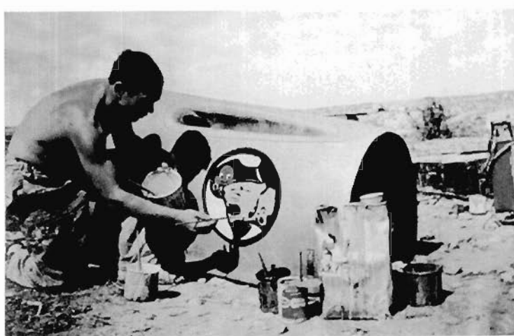
ABOVE: Conditions for painting in the field as opposed to those in a factory environment are illustrated by this desert setting of a ground staff member applying the final touches to a JG 27 emblem on a Bf 109 F cowling. Four of the standard issue paint tins are visible, plus a food tin used to wash the brushes out using benzine from the very battered fuel tin.
