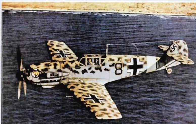
ABOVE AND RIGHT: In these two views, one of 'White 6', the other of 'Black 8' of 2./JG 27, the differences are again apparent. On the latter aircraft, the upper surface mottle had been carried down to the mid-line of the fuselage. The style of mottling on each aircraft was different.
