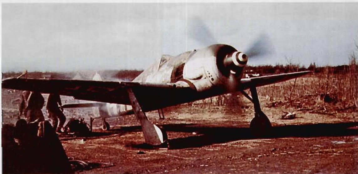
LEFT AND BELOW: These two colour photographs of the same aircraft help illustrate the overall finish of W.Nr. 681437. Note the starboard side of the engine cowling retains its original panel. This swapping of parts could produce some unusual camouflage effects. The black/white/black Reichsverteidigung markings were 900 mm wide. (Col. Leo C. Moon)
