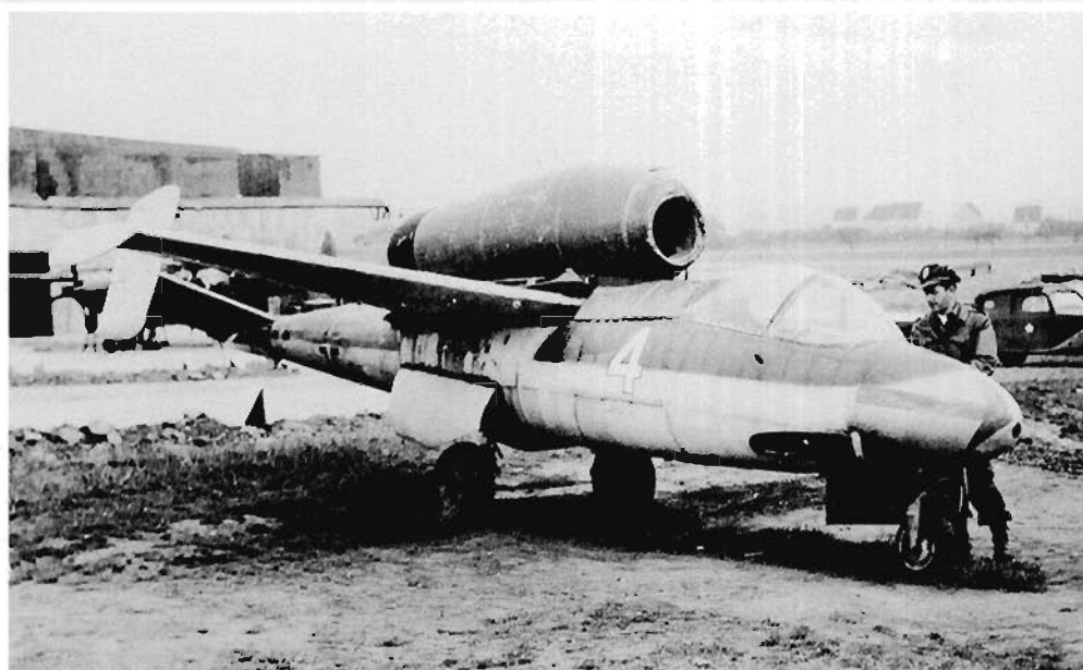
LEFT: The same machine, W. Nr. 120067 'Yellow 4' of JG 1, photographed under different light conditions after transfer to Kassel. Lack of O2-undercoat before application of the single coat of each camouflage colour allowed the filler paste lines to show through at this angle, making an interesting comparison with the previous photograph. The arrow marking was applied in red RLM 23.
