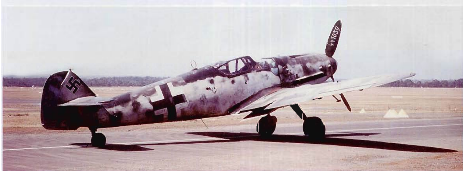
BELOW: This view of W.Nr. 163824 shows the 81/black-grey camouflage as well as the reduced amount of mottle on the fuselage side surface compared with that of the starboard side. The white number '441039' on the broad-blade VDM 9-12159 A propeller is the Werknummer of another Bf 109 G-6 that had surrendered its recycled propeller to this machine. This illustrates how parts were identified for the rebuilding cycle of each individual machine.
