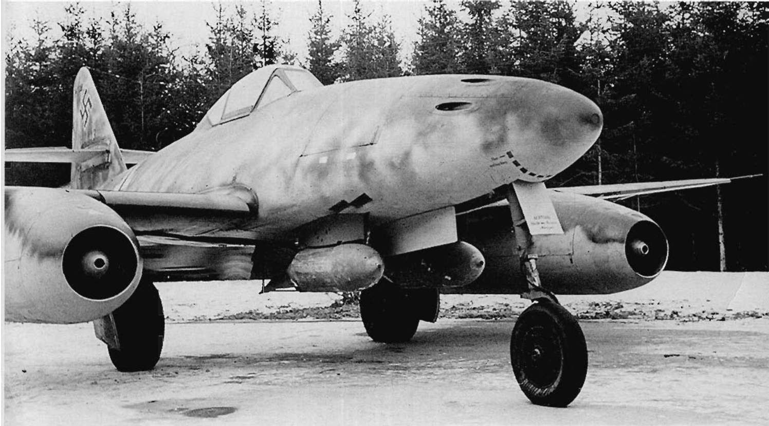
ABOVE: Me 262 A, W.Nr. 110813, had been used as a development aircraft for bomb trials in mid-1944. The two 250 kg bombs are mounted on Wikingerschiff bomb racks. Later, the aircraft served with Kommando Nowotny as 'Green 3'. Camouflage is 74/75/76, with a high demarcation line between upper and side surface colouring.
