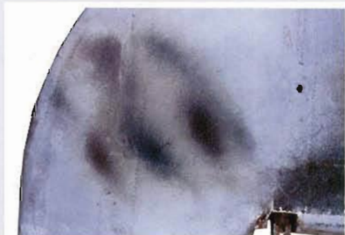
ABOVE: A close-up detail of the sprayed 83 on the rudder showing the coarse application caused by using too low a pressure with the spray gun.
