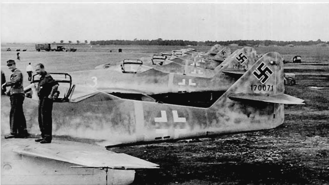
LEFT: A line-up of Me 262 A-1a's of Erprobungskommando 262 at Lechfeld in 1944, illustrating the close conformity of style of application of the 74/75/76-colouring, with soft mottling between the upper solid camouflage and the side surfaces. There are two patterns present, the A and B form mirror images of each other; the first and third aircraft have one form, the second and fourth the other (detail is too poor to determine what the remainder wore). This was normal, RLM approved practice at some production centres. The first two aircraft were W.Nr. 1700071 and 170067; all wore the narrow yellow 04-coloured fuselage band marking common to the unit's aircraft.
