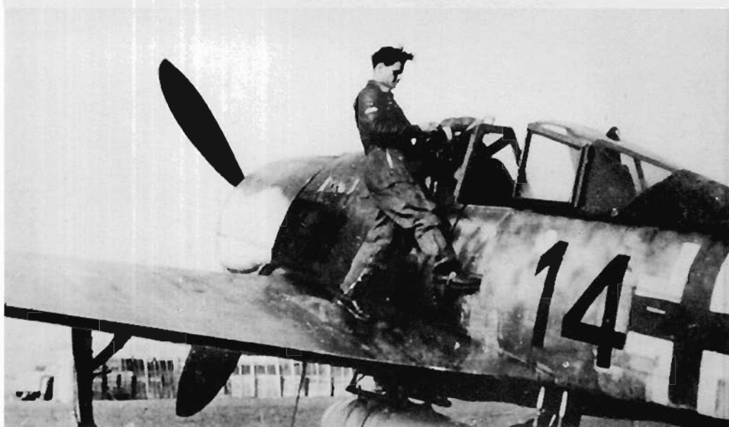
LEFT: A most unusually modified camouflage. The fuselage of the Fw 190 appears to be finished in a base coat of 82 with long thin patches of 81 added in semi-linear fashion. The fin and rudder lack anything but the 82-colouring, but around the Hakenkreuz the original 76 can still be detected. In contrast the wings and engine cowlings appear to be in very dark colours; possibly a much denser application of 81 and 82. (J. Crow)
