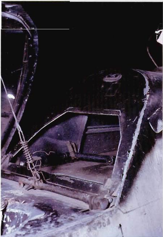
ABOVE: The rear section of the cockpit of Bf 109 G, W.Nr. 163824, showing the external non-standard black-grey camouflage colour which however substituted reasonably well for the regulation 66 in this instance. A very thin, roughly sprayed coat of the dark colouring had also been used inside the locker space.
