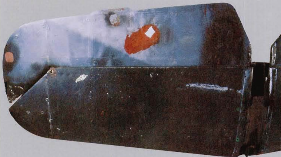
LEFT: The starboard tail plane upper surfaces with low contrast 81/83 finish on the fixed stabiliser and 74/75 on the recycled elevator. Note the crude repairs using the unidentified black-grey colour.
