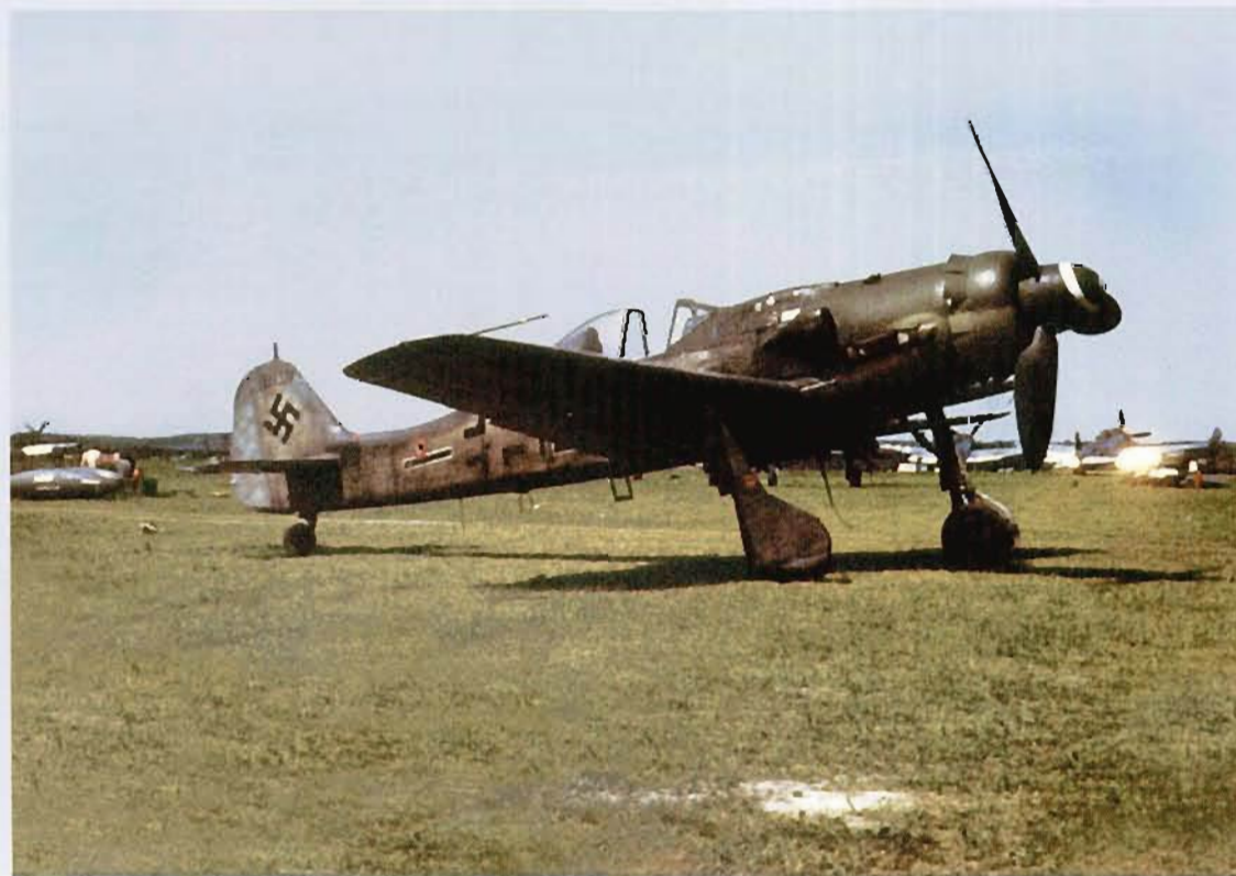
LEFT: Fw 190 D-9, W.Nr. 500571, 'Black 12' at Fürth at the end of the war. The main airframe was camouflaged in 81/82/76, but the 76 side surfaces had been toned down with a thin, sprayed coating of 02. The engine cowlings, which were supplied with the engine as part of the complete power unit, had a solid application of 82 on the upper surface and the unidentified green-blue colouring on side and lower surfaces. The colour difference is best assessed by comparing the 76 of the rudder with the area around the exhaust stubs on the engine cowling. While some aspects of the chemistry in 76 changed with a partial shift to use of Hansa blue in place of Cobalt blue very late in the war, it required long exposure to produce a greenish tinge to the colour – and the attrition rate did not favour such a time factor in many cases.
