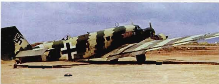
ABOVE: The break-up using 79-colouring to the dark greens of the European camouflage for flying over water is shown here to good effect; the ragged edges adding to the effectiveness of the camouflage. The background colour appears to be a single shade of brownish-green, but closer examination, particularly of the elevator, shows it to be standard 70/71 finish. The narrow 'white' band around the fuselage was the tactical marking for Luftwaffe forces based in the Mediterranean area and the narrowness may have been the strict interpretation of the 50 cm dimension set for the Bf 109 units. Ju 52 4U+NH was a unit hack operated by 1.(F)/123 in support of its Ju 88 force.
