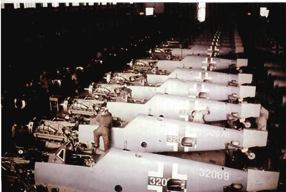
LEFT: Bf 109 G-6 production at Messerschmitt's Erla plant at Leipzig in the Autumn of 1943 shows fuselage structures painted in 76-overall with Balkenkreuz markings applied. Note the application by stencil of each airframe's Werknummer, in two places; the one across the Balkenkreuz required repainting of the black area of the marking later, but the other number would disappear beneath the upper surface camouflage greys of 74 and 75. The aft section, bolted to Frame 9, was a sub-contract component delivered in 02.
